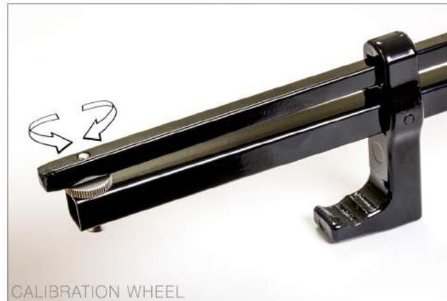
The fine tuning of your KEGCHECK is a quick and easy process, and is achieved by making slight adjustments to the calibration wheel. Simply turn the wheel clockwise, or anti-clockwise, to make a small adjustment to the rod spacing. Place back on the keg and follow the correct KEGCHECK measuring process. Repeat as necessary until the pointer on the measuring scale of your KEGCHECK handle accurately indicates the amount of a genuinely full keg.
