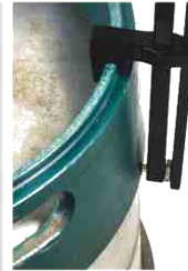
1 Position KEGCHECK on the rim of the keg
