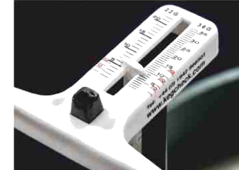
4. Record the measurement on the kegcheck scale in your stocktaking application.
